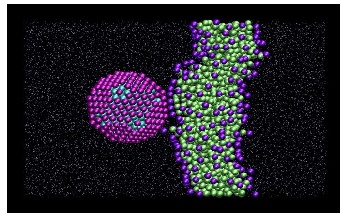
Molecular dynamics simulation setup to probe the interactions between a nanoparticle and a polymer strand in aqueous solution. The system size is 15 nm. A. Sambasivam & R. Sureshkumar (2012)
