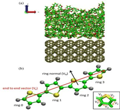
Snapshot of simulation box used to investigate OPV materials. Fullerene molecules are shown in dark green, on top of which oligothiophene molecules are adsorbed. (b) Snapshot of a single oligothiophene molecule in detail, showing the four rings for each molecule. The sulfur atoms are colored yellow, carbons are green, and hydrogens are gray. <u>http://pubs.acs.org/doi/full/10.1021/jp212548r</u>
