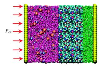
Water desalination through a nano (ZIF-8) membrane. Two chambers are separated by the ZIF-8 membrane: the one on the left is 0.5 M NaCl aqueous solution and the other on the right is pure water bath. An external pressure is exerted on the left chamber to mimic a reverse osmosis process.
