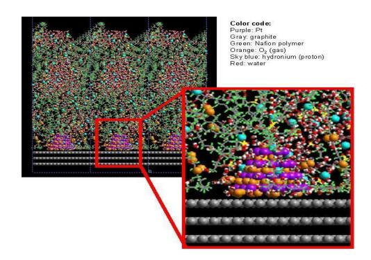
Model for simulating the Platinum/Nafion Interface in a Polyelectrolyte Membrane Fuel Cell. <u>http://www.wag.caltech.edu/fuelcells/projects/Nafion.html</u>
